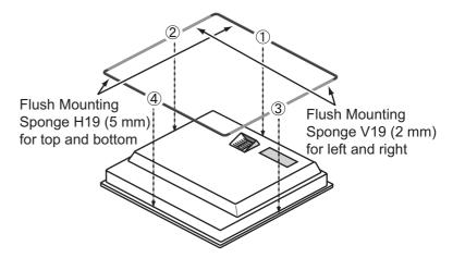
3. Attach the flush mount panels 19 to the monitor unit from the rear with the binding head screws (M4x10, 6 pcs., supplied).
